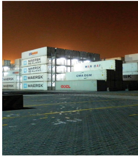
Figure 3. Container yard in an APM terminal in Mumbai, India showing the importance of uniform illumination on horizontal surfaces for navigating around the area and vertical surfaces for identifying tall stacks of containers. Installation and photo courtesy of EcoLights.
